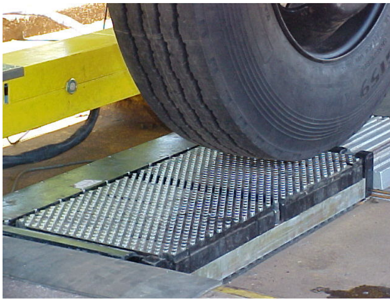
Figure 5: Single SIM pad configuration (used under Heavy Vehicle Simulator (HVS) with single test tyre).
