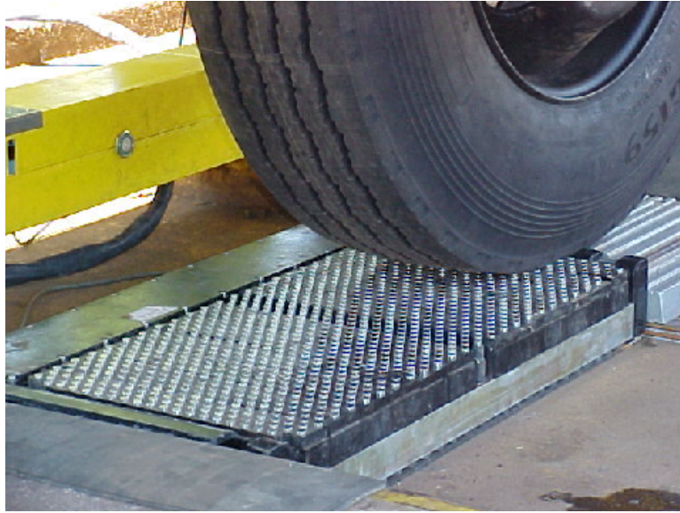
Figure 1: Single SIM pad configuration (used under Heavy Vehicle Simulator (HVS) with single test tyre).
