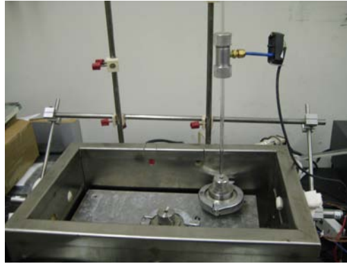
Figure E2d.1. New dilatometric testing system.
