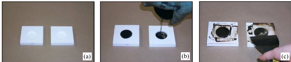
Figure M2c.1. Photo. (a) Prepare clean silicone molds. (b) Pour the molten binder. Let the binder to cool down to room temperature (approx. one hour). (c) Dress the binder with a heated putty knife (Picture by Kitae 2005).
