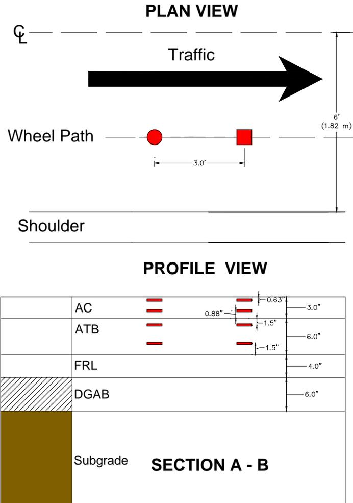
Figure V3c.3. Detail of rosettes instrumentation for Sections A and B.
