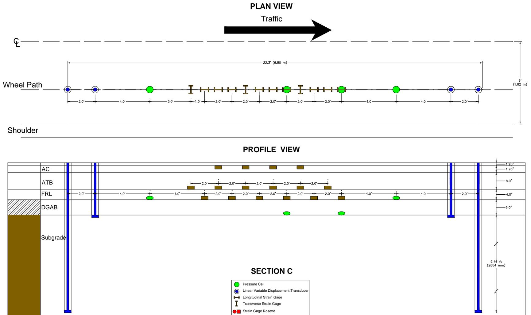
Figure V3c.2. Pavement structure and instrumentation of Section C (15-in-thick).
