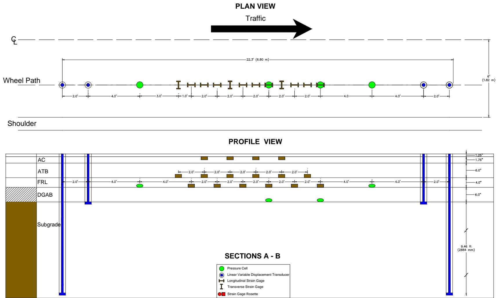
Figure V3c.1. Pavement structure and instrumentation of Sections A and B (13-in-thick).
