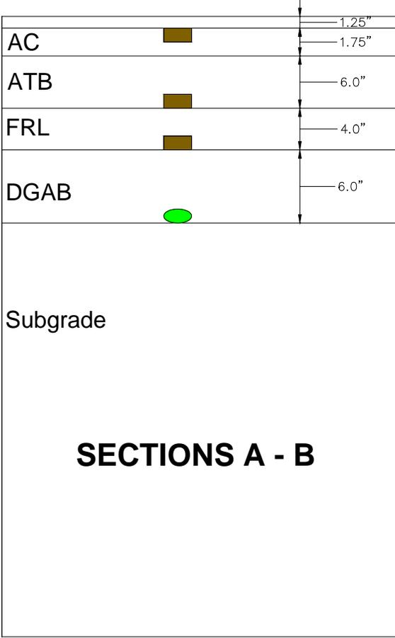
Figure V3c.5. Cross section of pavement structure and instrumentation for Sections A and B.
