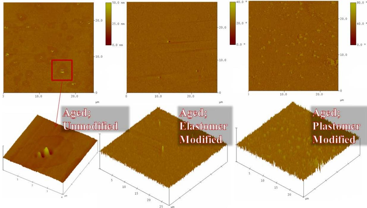
Figure F2d.4: Effects of polymer modification on asphalt aging (25  $\mu\text{m}$  by 25  $\mu\text{m}$  AFM topography/phase images).
