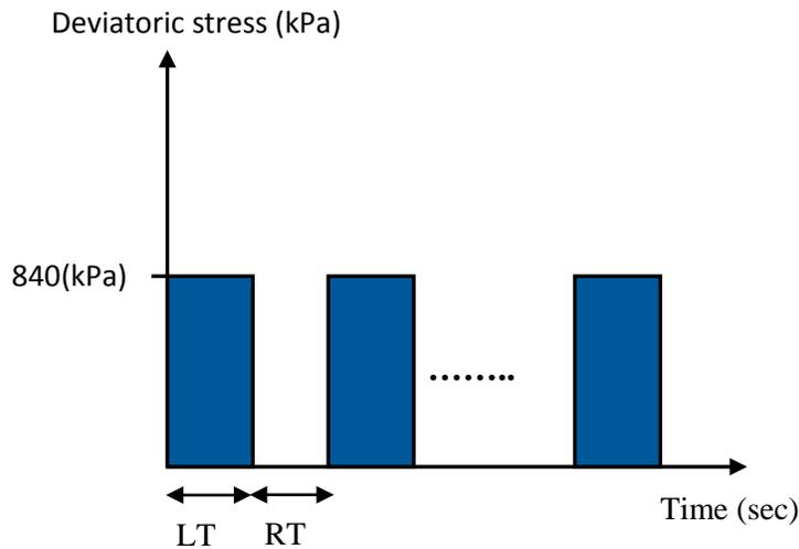
Figure V3c.A.2. Schematic representation of the stress input for RCRT-CLR test. Both loading time (LT) and resting time (RT) are constant through the entire test.
