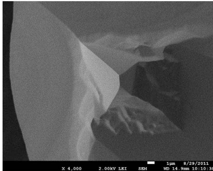
Figure F2d.5. Scanning electron microscope image of AFM tip used in this study.
