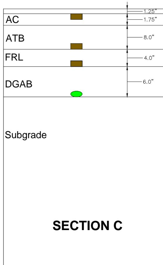
Figure V3c.6. Cross section of pavement structure and instrumentation for Section C.
