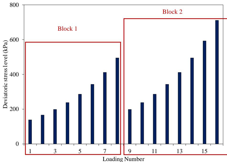
Figure V3c.A.1. Stress history for the RCRT-VS test.
