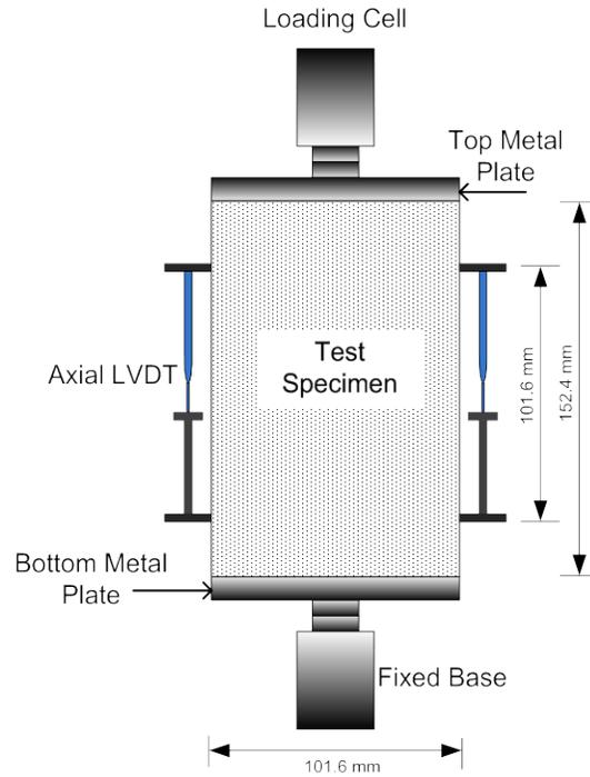
Figure V3c.A.6. Schematic view of test setup with Mounted Axial LVDTs.
