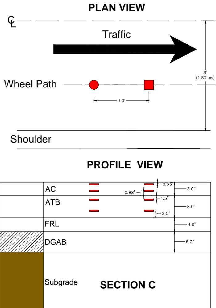
Figure V3c.4. Detail of rosettes instrumentation for Section C.
