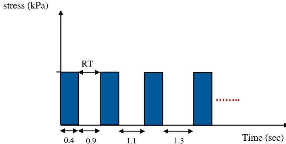
Figure V3c.A.3. Schematic representation of the stress input for RCRT-VRT test. Loading time (LT) remains constant through the entire test where the resting time (RT) changes for each loading cycle.
