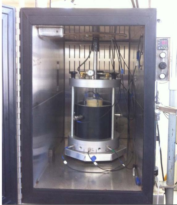
Figure V3c.A.5. Tri-axial Cell inside Environmental Chamber.
