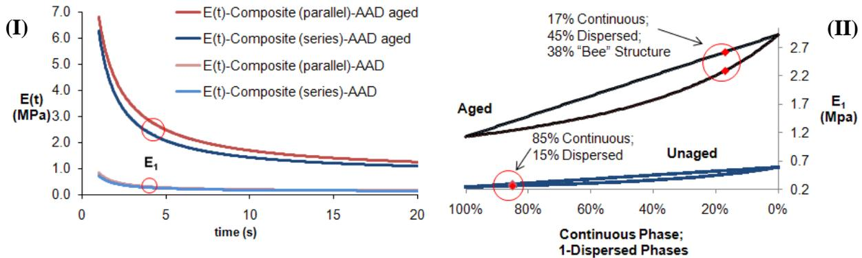
Figure F2d.3. (I) Bounds for the composite relaxation modulus  $[E(t)]$  of unaged and aged asphalt AAD and (II) the relationship between individual phase modulus, phase distribution, and composite  $E(t)$  values.
