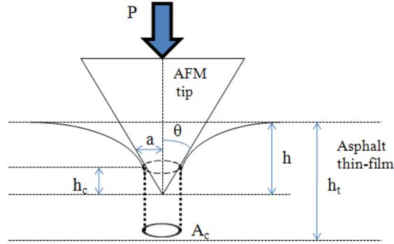
Figure F2d.2. Geometry of AFM indentation test.  $P$  is the indentation load,  $h_t$  is the asphalt film thickness,  $h$  is the indentation depth,  $h_c$  is the contact depth,  $A_c$  is the projected contact area, and  $a$  is the contact radius (Adapted from Vandamme [1]).
