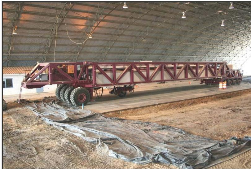
Figure V3c.7. Heavy Vehicle Simulator used to apply loading repetitions.
