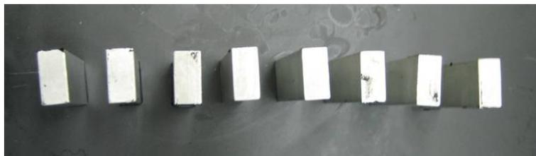
Figure E2d.9. Adhesion issues with PPA-modified Flint Hills binder.
