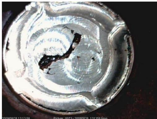
Figure M2c.1. Photograph. Asphalt/pull-out stub failure on the stub with legs.
