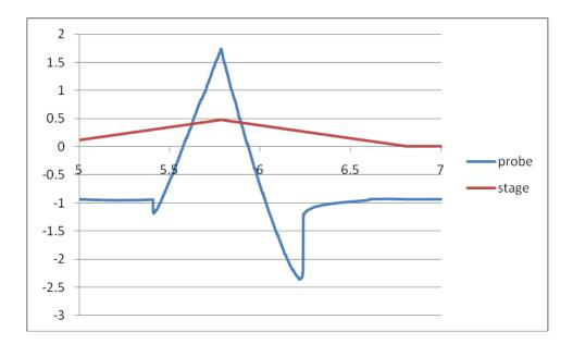
Figure M2a-2.2. FDC (as collected) for SHRP core asphalt AAA-1 at ambient temperature.
