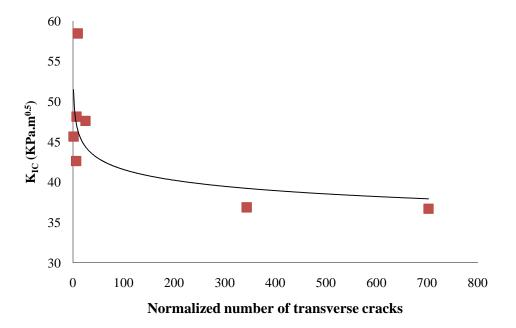
Figure V3b-3.1. Graph. Fracture toughness at -24°C vs. normalized number of transverse cracks on LTPP sections.
