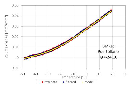
Figure E2a.1. Graph. Glass transition temperature for BM-3c- Puertollano binder.
