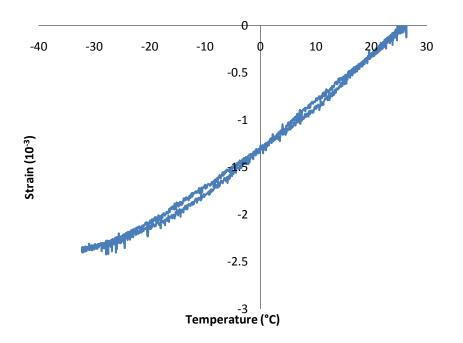
Figure.E2d.7. Thermal strain for MnROAD Cell 20 sample during one cooling and heating cycle.
