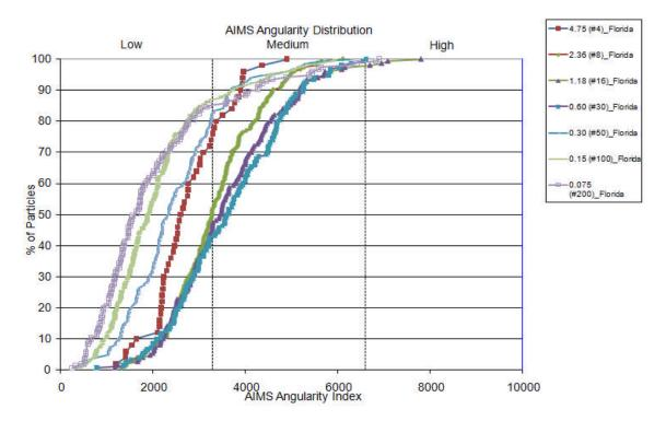
Figure E2c.5. Aggregate angularity for FLDOT aggregate source.
