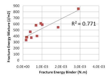
Figure E2a.2.Graph. Correlation between binder and mixture fracture energy.
