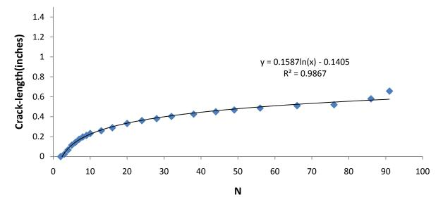
Figure E1a.10 shows the calculated crack growth for a specimen of which the values of  $E_1$  and m are 47544 psi and 0.351, respectively.
