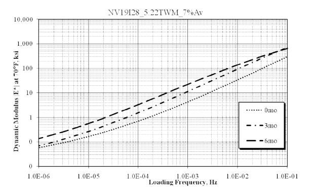
Figure E2d.3. Dynamic modulus tensile creep.
