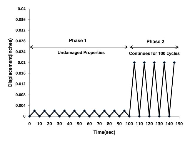
Figure E1a.8. OT test loading pattern.
