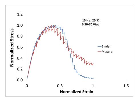
Figure E2a.4. Graph. Mixture (EBADE) and binder (LAS) normalized stress-strain response to accelerated fatigue.
