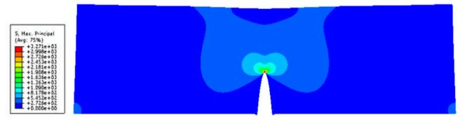
Figure E1a.4. Principal stress distribution in deformed specimen with loading displacement of 0.025 inches and crack length of 0.625 inches.
