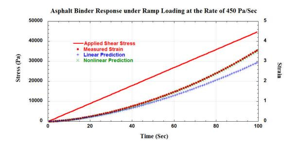
Figure F1b-1.2. The comparison of model predictions and laboratory measurements for asphalt binder PG 76-22 under ramp loading with the rate of 450 Pa/Sec at 28°C. Where  $N_1$  is the first normal stress difference.
