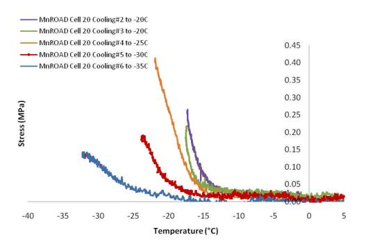
Figure E2d.5. Stress buildup curves under thermal cycling for MnROAD Cell 20.
