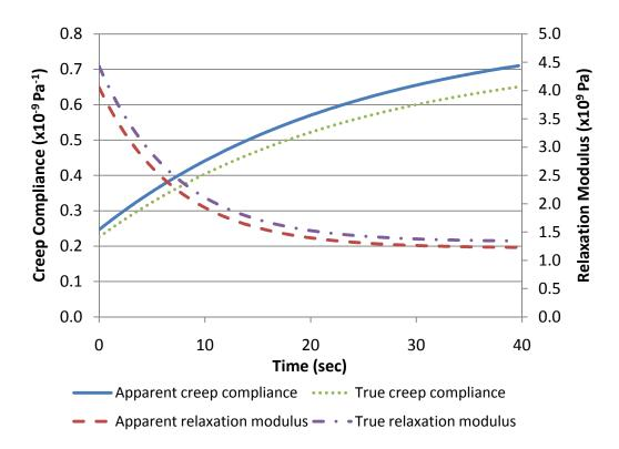
Figure E1a.1. Apparent and true material properties of undamaged asphalt mixtures.
