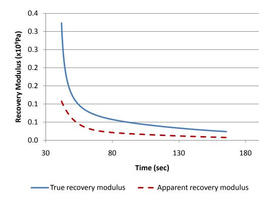
Figure E1a.2. Apparent and true recovery modulus.
