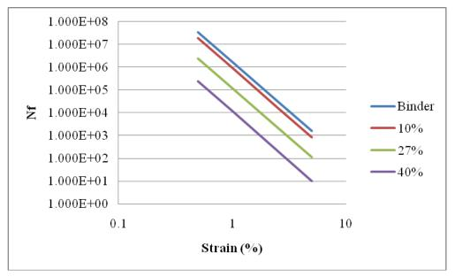
Figure F2e.3. Graph. Effect of filler volume fraction on relationship between number of cycles to failure (Nf) and strain.
