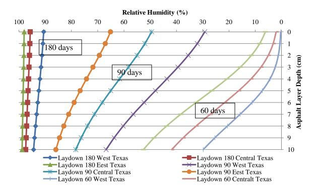
Figure E1a.11. HMA layer relative humidity modeling.
