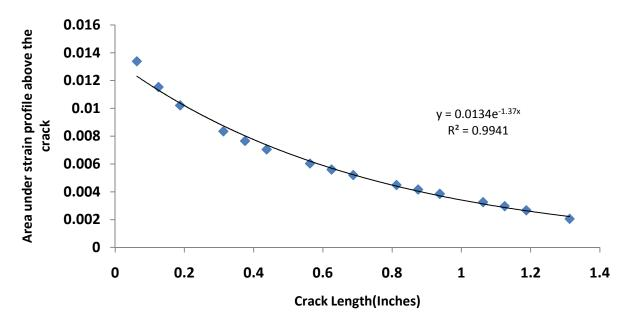
Figure E1a.9. The crack length versus the integration of strain profile above the crack.
