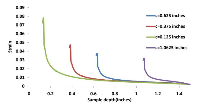
Figure E1a.5. Strain profiles above crack tip when crack size is 0.125, 0375, 0.625 and 1.0625 inches, respectively.
