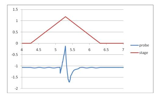
Figure M2a-2.3. FDC (as collected) for SHRP core asphalt AAA-1 at 44° C.
