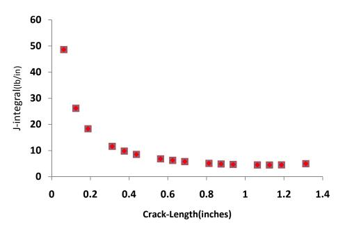
Figure E1a.7. J-integral versus crack length.
