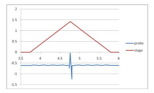
Figure M2a-2.4. FDC (as collected) for SHRP core asphalt AAA-1 at -4° C.
