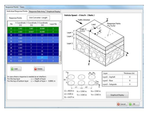
Figure VP3a.1. Input window for Individual Response Points if static and performance analysis is selected.
