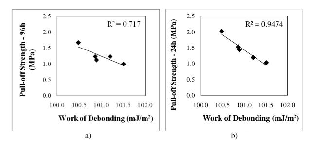
Figure M1a.3. Graph. Comparison between pull-off strength and work of debonding of binders with adhesive failure with granite after a) 96 hours and b) 24 hours of conditioning.
