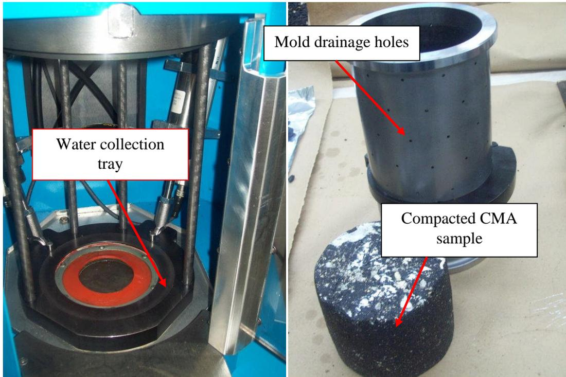
Figure E1c-2.1. Photograph. Modified gyratory mold and apparatus with compacted CMA sample.
