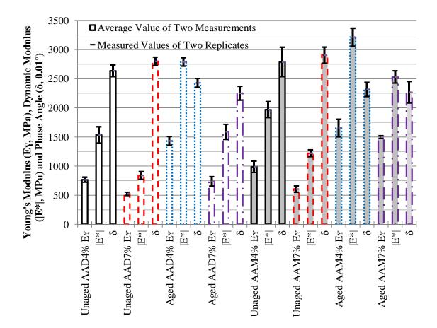
Figure F2c.1. Young's modulus, dynamic modulus and phase angle for different asphalt mixtures at 40°C.
