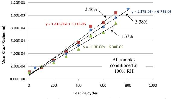
AAM34\_RH100\_Air Void 3.46% AAM23\_RH 100%\_Air Void 3.38% AAM10\_RH100\_Air Void 1.37%
