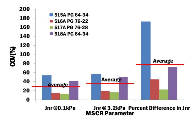
Figure V3a.1. Coefficient of variation of the MSCR results for data collected from more than 25 labs.
