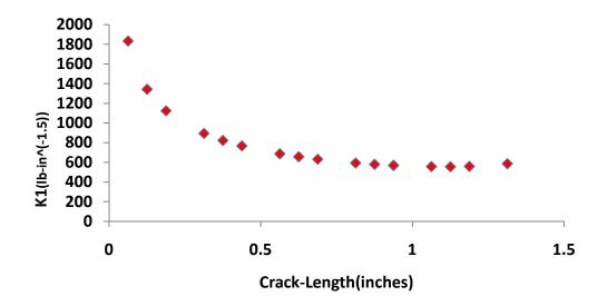
Figure E1a.6. The stress intensity factor versus crack length.
