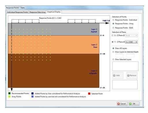
Figure VP3a.3. Graphical display for Array Points on Y-Z plane.
