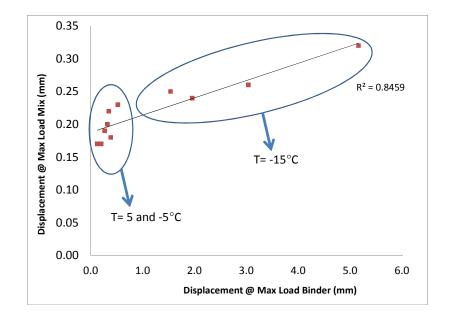
Figure E2a.3. Graph. Displacement at maximum load in mixture and binder in low temperature cracking testing.
