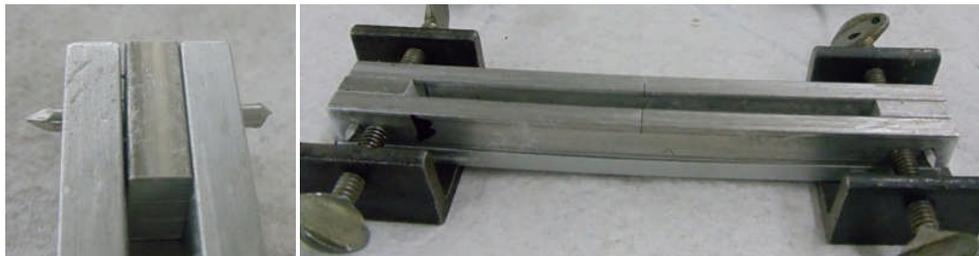
Figure E2d.2. Modified SENB mold system with alignment pins.
