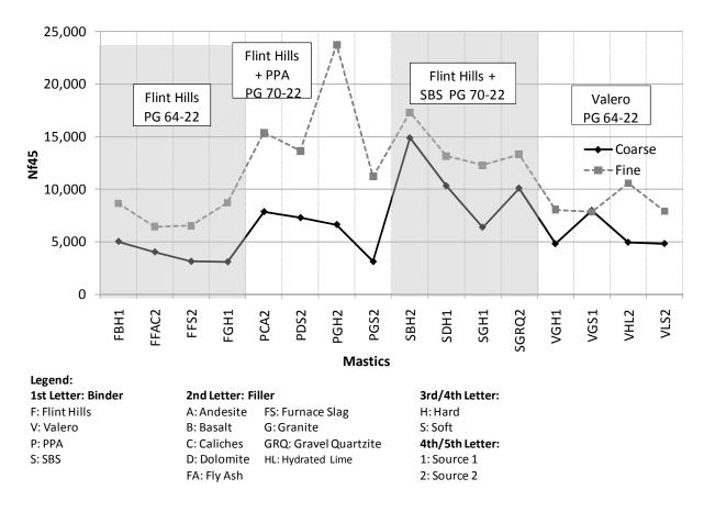
Figure F2e.1. Graph. Mixture IDT fatigue results from NCHRP 9-45 (Bahia et al. 2011).
