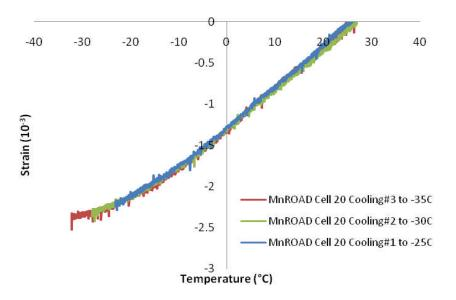
Figure E2d.6. Graph. Thermal strain in MnROAD Cell 20 in the cooling cycles.
