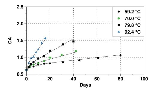
Figure F1c-3.1. Comparison of model calculations (solid lines) of CA to experimental data (symbols) for NuStar PG 67-22.
