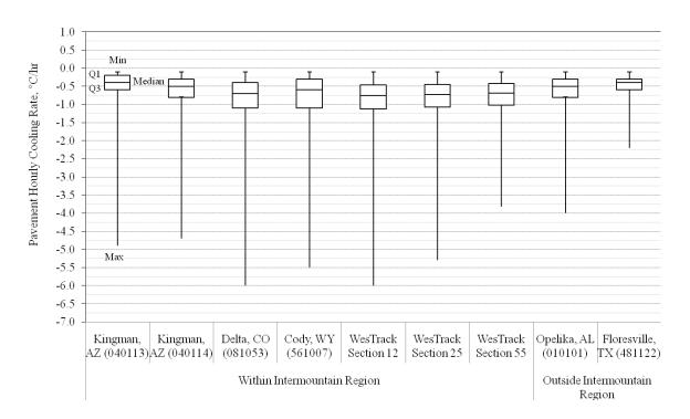
Figure E2d.1. Box plots of all sections at a sensor depth of approximately 12.5 mm using hourly cooling rate data from pavement temperatures of 10°C or colder categorized by region.
