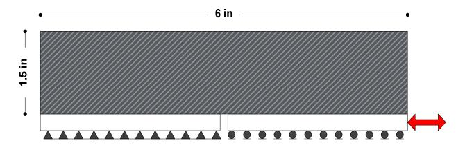
Figure E1a.3. Overlay tester setup and boundary conditions of the finite element model.
