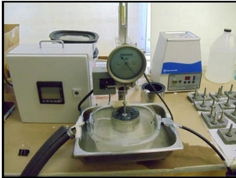
Figure E1b-2.1. Photograph. Modified temperature controlled indentation/penetration test.
