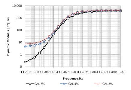
Figure E2c.3. Dynamic modulus at 20°C for Granite (West California).
