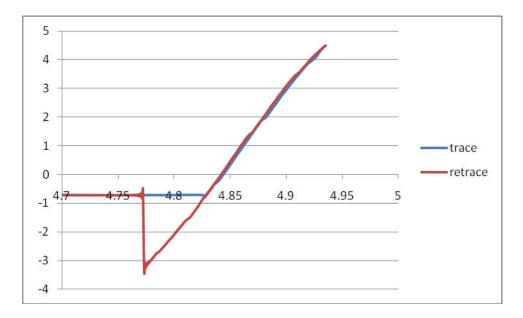
Figure M2a-2.1. A typical example of a FDC collected on a glass substrate using the modified AFM/nano-positioning stage system.
