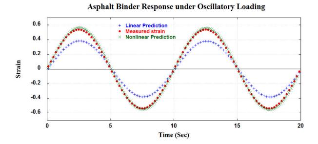
Figure F1b-1.1. The comparison of model predictions and laboratory measurements for asphalt binder PG 76-22, at 48.1 kPa shear stress level, 0.1 Hz, and 28°C.
