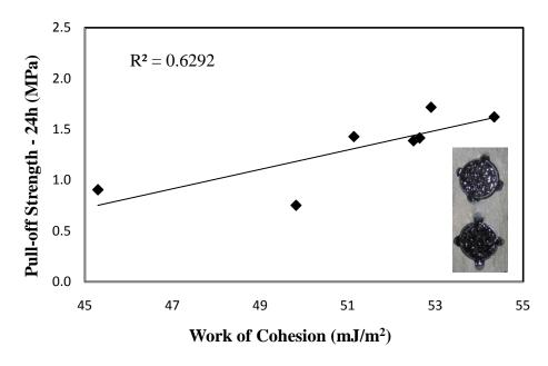
Figure M1a.1. Graph. Comparison between pull-off strength and work of cohesion of asphalt binders that showed cohesive failure with limestone aggregate after wet conditioning.
