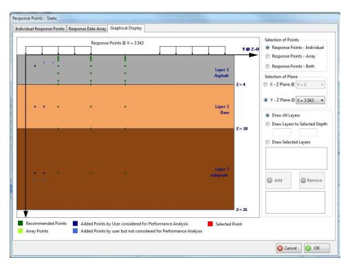
Figure VP3a.2. Graphical display for Individual Response Points on Y-Z plane.
