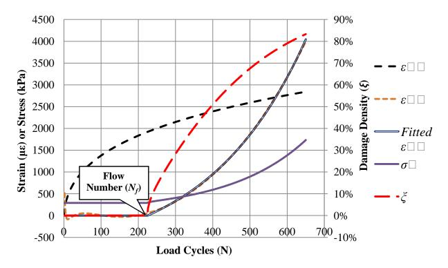
Figure F2c.3. Viscoplastic strain, viscofracture strain, true stress and damage density.
