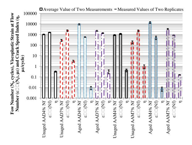
Figure F2c.2. Flow number, viscoplastic strain at flow number and crack speed index for different asphalt mixtures at 40°C.
