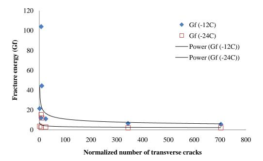
Figure V3b-3.2. Graph. G<sub>f</sub> vs. normalized number of transverse cracks at -12°C and -24°C.
