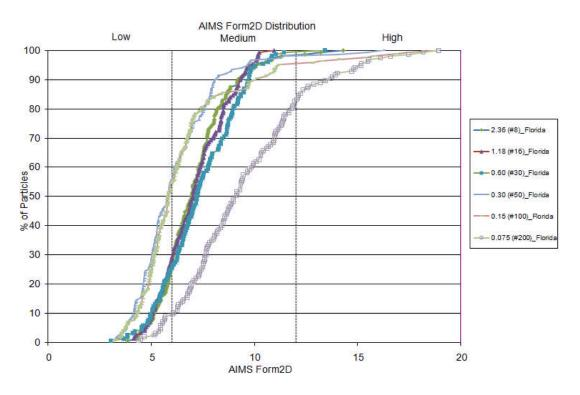
Figure E2c.4. Aggregate form for FLDOT aggregate source.
