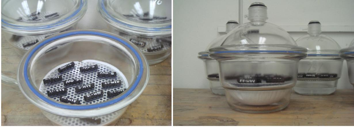
Figure E1a.8. DMA specimens conditioning in desiccators.
