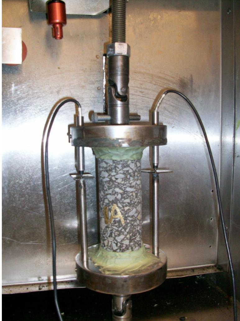
Figure E2d.7. Cylindrical specimen in the TSRST chamber.
