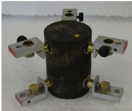
Figure E1a.12. Configuration of creep test on limestone soaked in AAD binder.
