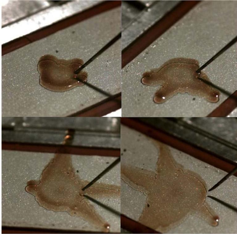
Figure M1b-2.10 cont. High speed video images showing the time lapse of a developing spin cast film as fingering instability develops (late).
