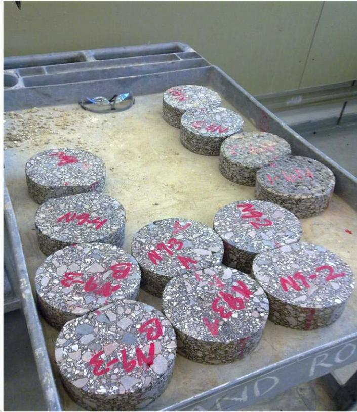
Figure F1c-4.4. Typical cores of asphalt surface layers.
