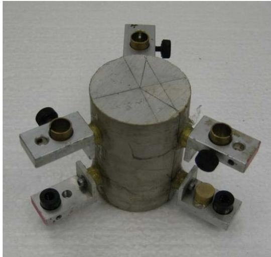
Figure E1a.11. Configuration of creep test on fresh limestone sample.
