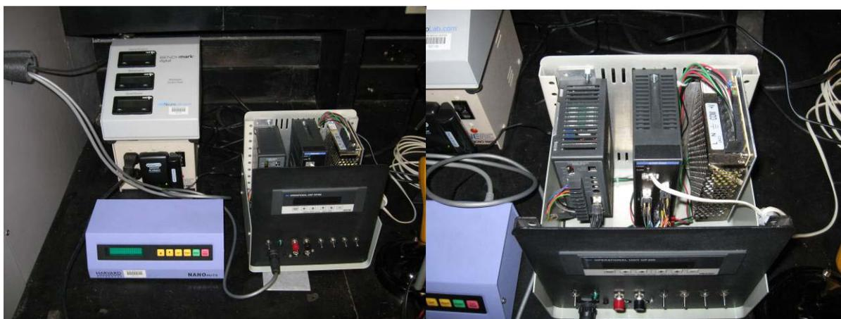
Figure M1b-2.9. Controllers for robotic arm and nano-syringe pump.
