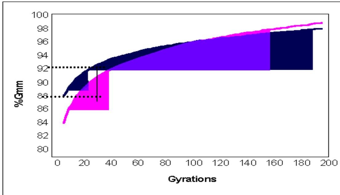
Lower Compactive Effort is recognized by a smaller area under the compaction curve from 88 – 92% Gmm
