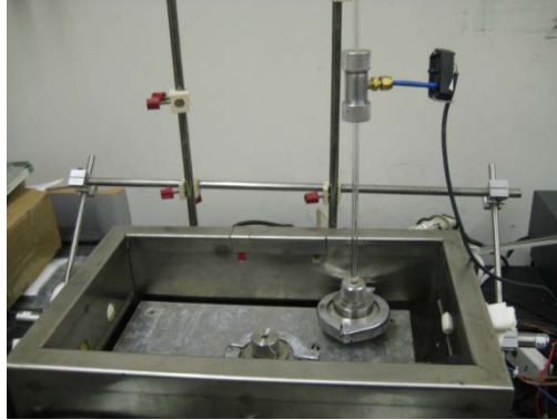
Figure E2d.1. New dilatometric testing system.
