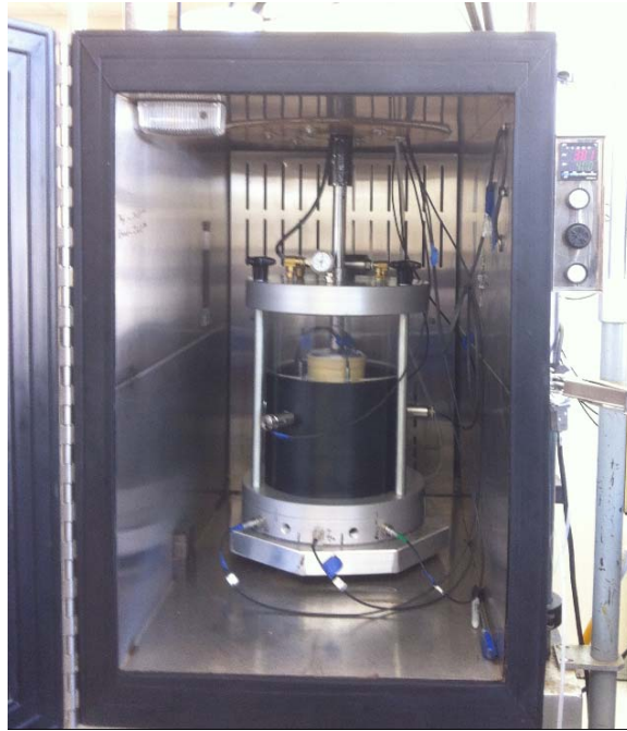
Figure 5. Tri-axial Cell inside Environmental Chamber.
