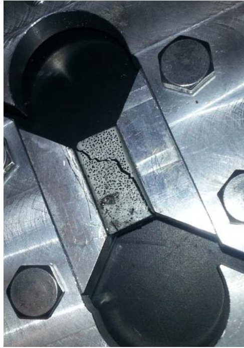
Figure F1b.1. Illustration of a failed FAM test specimen in the Arcan apparatus to identify limits of loading and loading rate; the Arcan apparatus is used to evaluate material response under multi-axial stress states.
