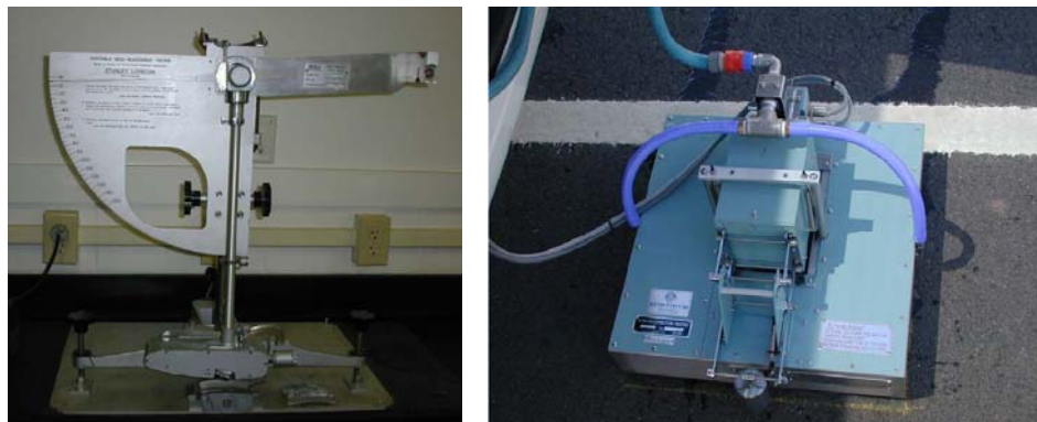
Figure VP2.1. Photos. Skid resistance measurement devices: British pendulum and dynamic friction tester (Image source: Brown et al. 2001).
