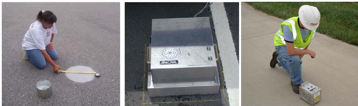
Figure VP2.2. Photos. Asphalt pavement texture measurement techniques: sand patch method, circular texture meter, and Ames texture scanner (Image sources: Hanson and Prowell 2004). Ames Engineering 2007).
