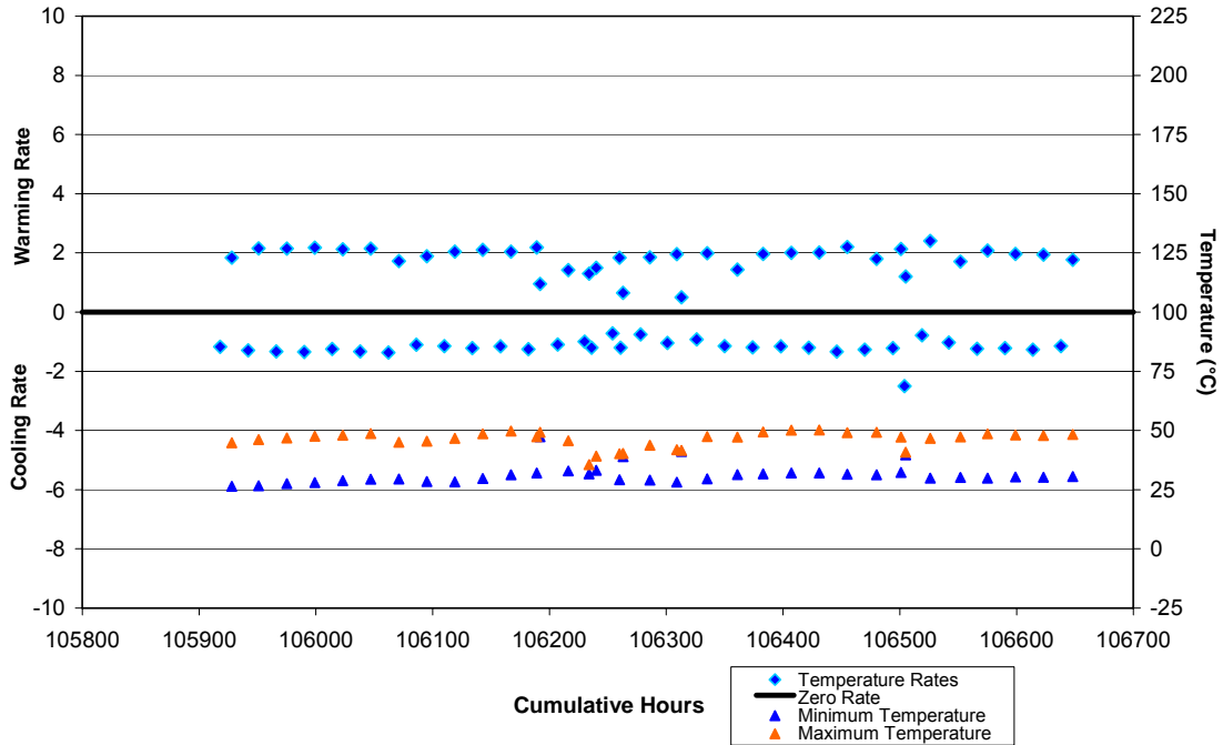
Figure E2d-1.9. Pavement temperature rates along with the maximum and minimum daily temperatures for test section 040113 at sensor 2 (depth = 2.9 inches) for July of 2004.
