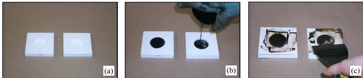
Figure M1a.1. Photos. (a) Prepare clean silicone molds. (b) Pour the molten binder. Let the binder to cool down to room temperature (approx. one hour). (c) Dress the binder with a heated putty knife (Pictures by Kitae 2005).
