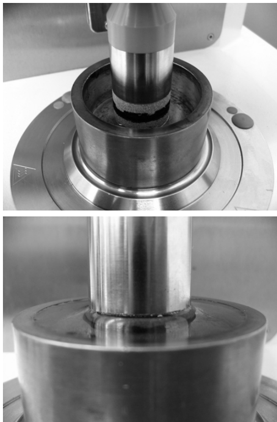
Figure M2c.1. Photos and charts. Representative data for the modified DSR test with wet and dry testing (SS = sandstone, LS = limestone).
