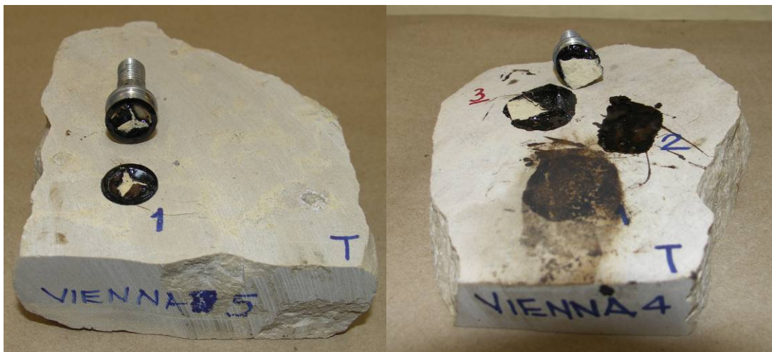
Figure M2c.4. Photographs. Example of pullout test failure at the rock. The Vienna rock source will not be used in future testing.
