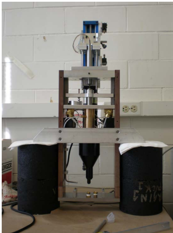
Figure E2d.3. Photograph. Assembled frame of the new BBR and SENB equipment.
