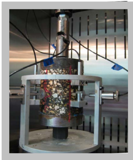
Figure F2c.1. Configuration of test protocol for viscoelastic characterization of asphalt mixture.
