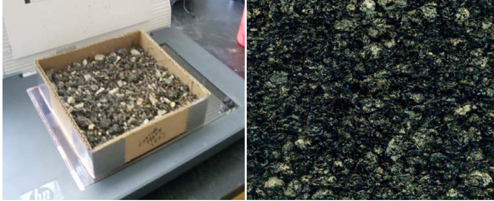
Figure E1c-2.1. Photograph. Coating analysis frame with CMA sample (left); scanned CMA image for CMA sample (right).
