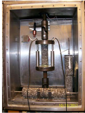
Figure E2d.1. Photo. TSRST set-up for measuring fracture properties and thermal strain.
