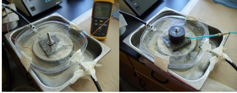
Figure M1a.2. Photograph. BBS test with controlled temperature.
