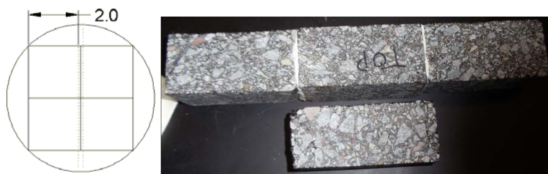
Figure E2d.2. Illustration and photograph. Prismatic beams made from gluing blocks cut out of gyratory-compacted samples.
