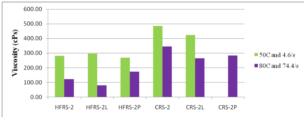
Figure E1c-2.3. Chart. Viscosity at a shear rate of 4.65/sec at temperatures of 50 °C and 80 °C for six emulsions.
