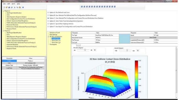
Figure VP3a.4: Axle configuration/contact pressure distribution, Option C (Tire Database)(ver. 3)
