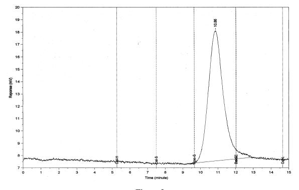
Figure 3 Example of Asphalt Without Polymer Modifier (0.2%) Concentration
