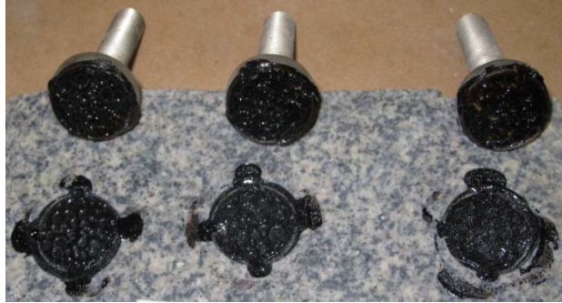
Figure M1a.1. Photograph. Cohesive failure for asphalt binder FH 64-22+0.5% anti-stripping with granite.
