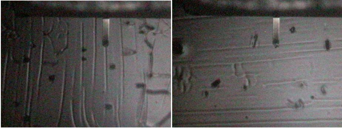
Figure F3a-8.5. AAA-1, photographed directly after freeze-fracturing (LEFT), and (RIGHT) after 30 days storage at ambient conditions ( \sim 7.6^{\circ}\text{C} ).
