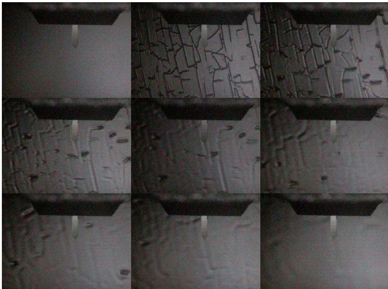
Figure F3a-8.1. AAG-1, photographed before and each day after freeze-fracturing for a total of 10 days, storage at ambient conditions ( \sim 25^{\circ}\text{C} ).
