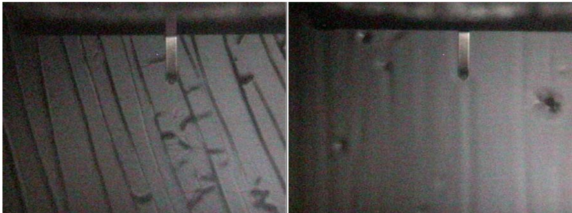
Figure F3a-8.6. AAD-1, photographed directly after freeze-fracturing (LEFT), and (RIGHT) after 10 days storage at ambient conditions ( \sim 25^{\circ}\text{C} ).
