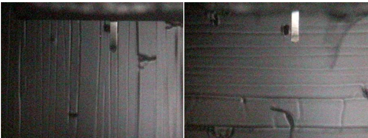
Figure F3a-8.7. AAD-1, photographed directly after freeze-fracturing (LEFT), and (RIGHT) after 30 days storage at ambient conditions ( \sim 7.6^{\circ}\text{C} ).
