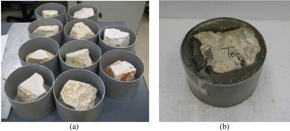
Figure E1a.1. Configuration of coring a cylindrical rock specimen.
