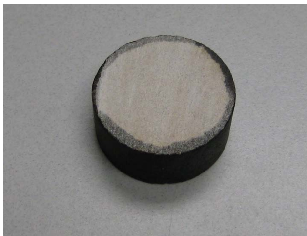
Figure E1a.4. Cross section of rock specimen after soaking in asphalt for 32 hours.
