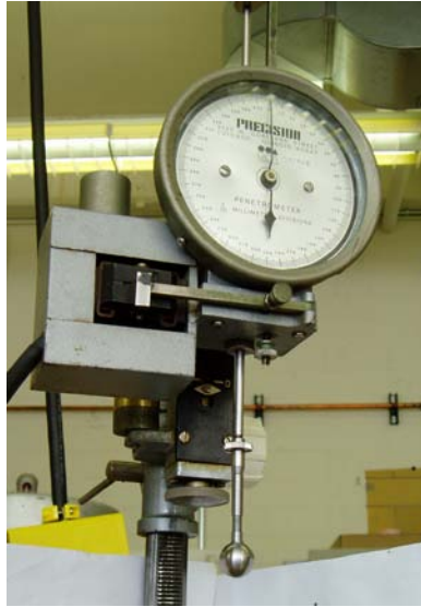
Figure E1b-2.3. Photograph. The indentation assembly showing the ball and the micrometer gauge.
