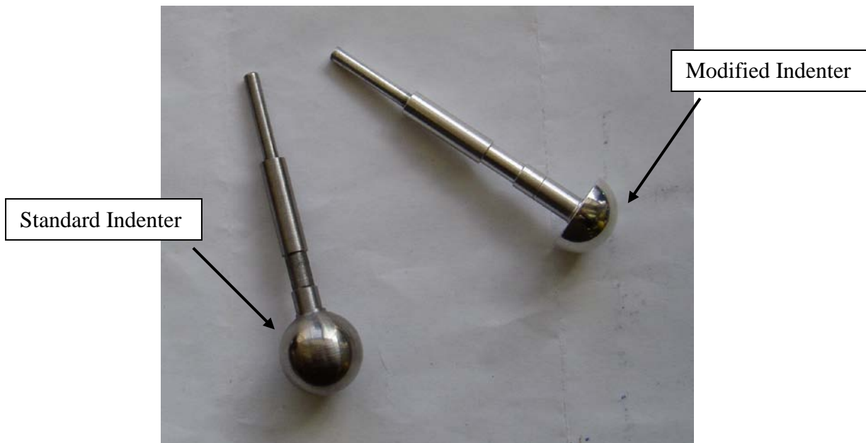
Figure E1b-2.4. Photograph. The standard indenter and the modified indenter.
