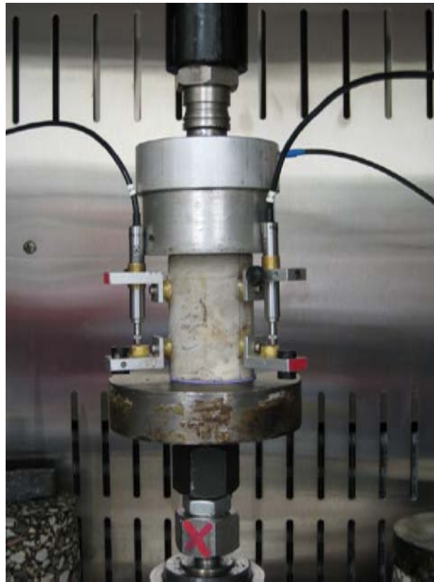
Figure E1a.3. Configuration of creep test on rock specimen.
