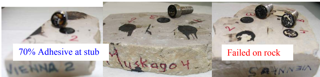
Figure M2c.7. Graphs and photographs. Pullout tension vs. deformation history: Elvaloy-modified binder on limestone surface with binding temperature of 65 °C and pressure rate of 870 kPa/s.
