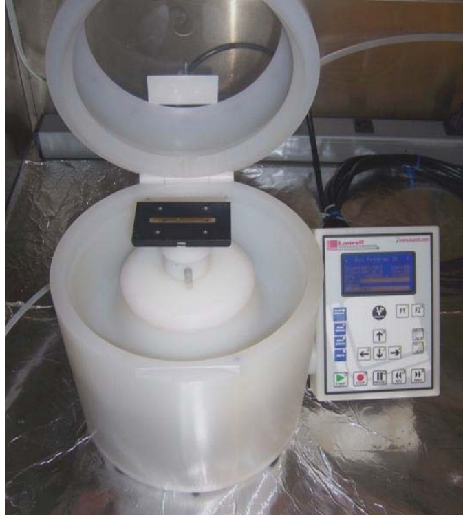
Figure M2b.1. Spin coater being used to cast thin films of the binder on a Zn-Se FTIR window.
